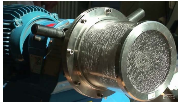
Figure 1: Transparent experimental grinding chamber of a high energy ball mill
