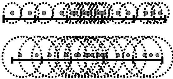
Figure 8: Illustration of the scanning window of two fixed lengths w=0.1 and w=0.2 . The centers of scanning windows are points with time coordinates t_1, t_2, \dots, t_N
