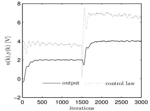
Figure 9: Evolution of the output and the control law (Case:  $PI - ISE$ )
