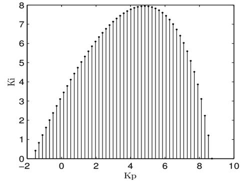
Figure 8: PI controller stability domain for  $PT - 326$
