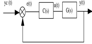
Figure 1: Closed-loop control of a time delay system
