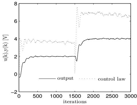
Figure 10: Evolution of the output and the control law (Case:  $PI - IAE$ )
