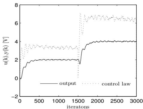
Figure 12: Evolution of the output and the control law (Case:  $PI - ITSE$ )
