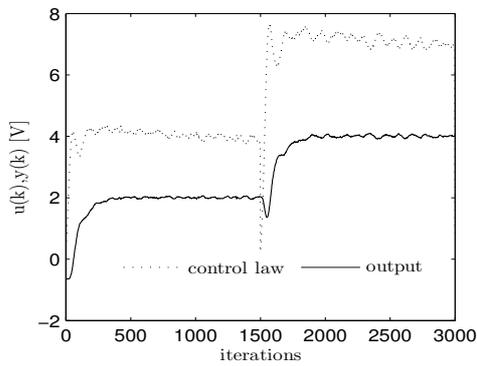
Figure 11: Evolution of the output and the control law (Case:  $PI - ITAE$ )
