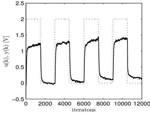
Figure 6: Square input 0V/2V and outputs of  $PT - 326$
