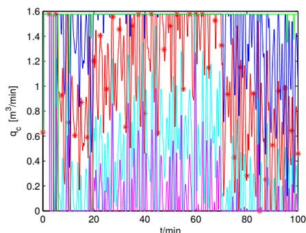
Figure 10: Robust PID stabilization of the CSTR with disturbances and noisy signals - control input  $q_c$
