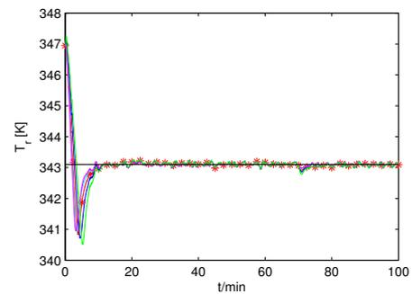
Figure 8: Robust PID stabilization of the CSTR with disturbances and noisy signals - controlled output
