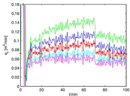
Figure 9: Robust PID stabilization of the CSTR with disturbances and noisy signals - control input  $q_r$
