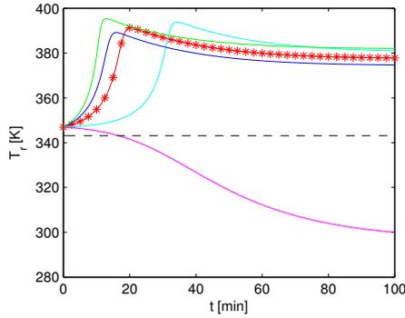
Figure 2: Open-loop response of the CSTR
