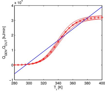
Figure 1: Multiple steady states of the CSTR
