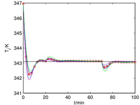
Figure 3: Robust PI stabilization of the CSTR - controlled output
