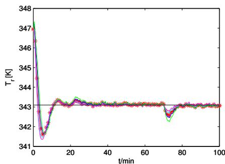
Figure 5: Robust PI stabilization of the CSTR with disturbances and noisy signals - controlled output
