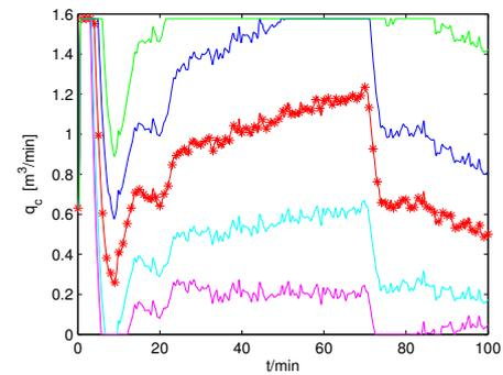
Figure 7: Robust PI stabilization of the CSTR with disturbances and noisy signals - control input  $q_c$
