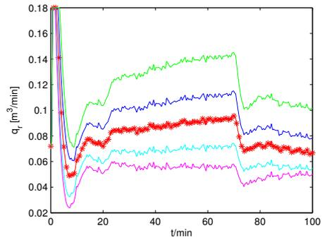
Figure 6: Robust PI stabilization of the CSTR with disturbances and noisy signals - control input  $q_r$
