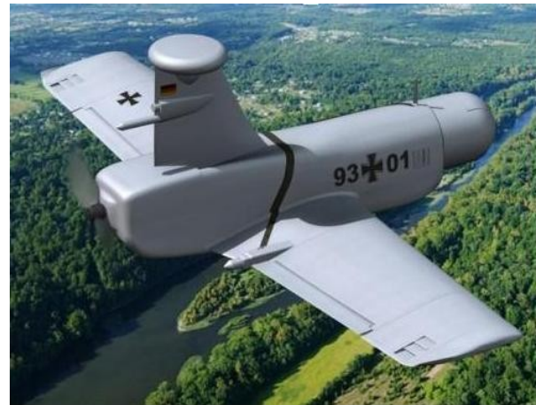
Figure 2. A Rheinmetall KZO of the German Army, used for target acquisition and reconnaissance (photo: Wikipedia)
