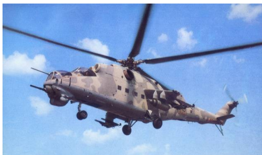
Figure 1. Mi-24 helicopter – example of armour integrated with fuselage of the helicopter (photo: Wikipedia)
