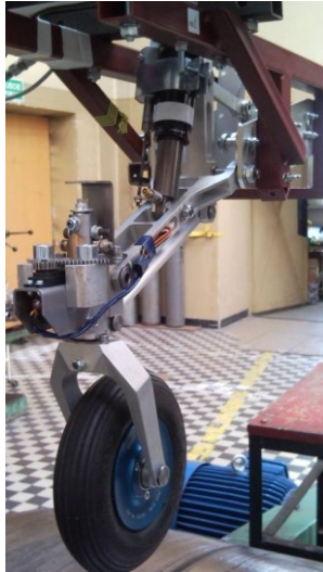
Figure 6. Nose Landing Gear on test stand in Laboratory (photo: IA archive)
