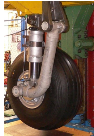
Figure 5. M-28 „Skytruck” main L/G with oleo-pneumatic shock absorber (design Institute of Aviation L/G Department, photo: IA archive)
