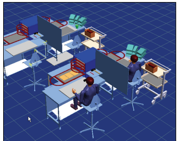
Fig. 3 – Modular design for two workstations used for producing leather goods.
