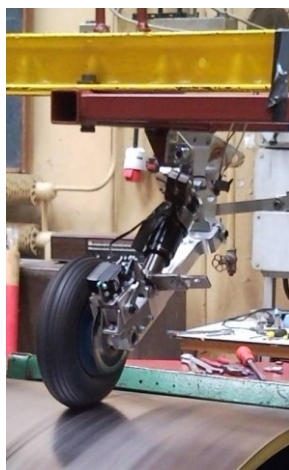
Figure 7. Main Landing Gear on test stand in Laboratory (photo: IA archive)
