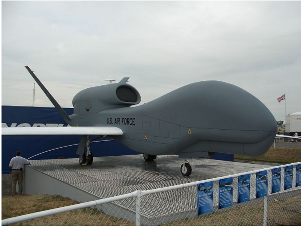
Figure 3. RQ-4 Global Hawk, a high-altitude reconnaissance UAV capable of 36 hours continuous flight time. (photo: Wikipedia)
