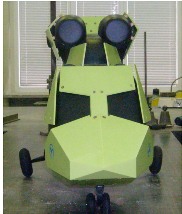
Figure 8. Front view of armour installed on helicopter model (model used in wind tunnel tests)
