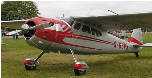
Figure 4. Spring beam L/G for Cessna 195 airplane (photo: Wikipedia)
