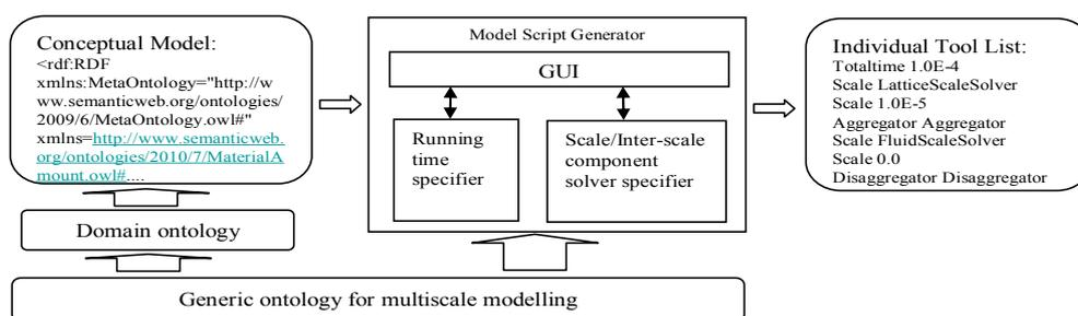
Figure 3: Design of the Simulation Script Generator (SSG)
