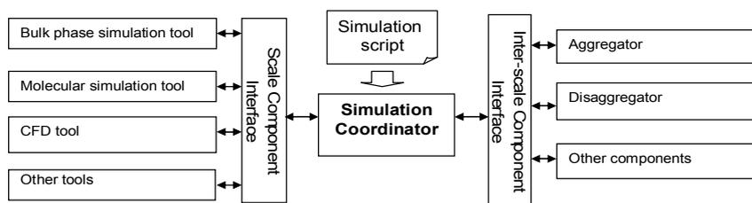
Figure 4: Design of the Model Execution System (MES).
