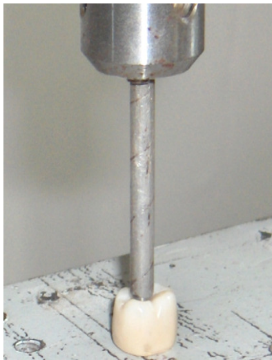
Figure 7: Centric compression of the composite material tooth sample
