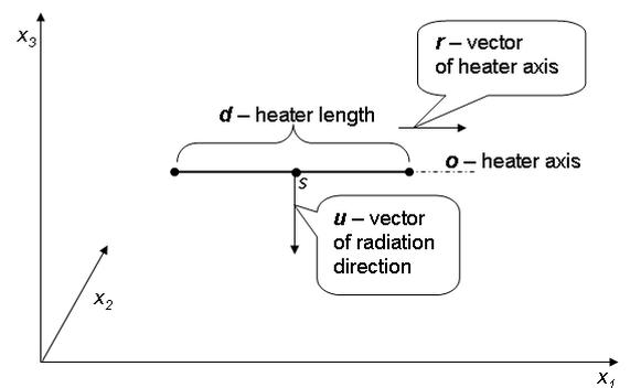
Figure 2: Representation of the Heater in the Model
