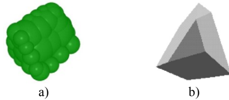
Figure 2: Examples for Modelling Rocks with Clumps (Coetzee and Nel 2014), and Polyhedra (Huang and Tutumler 2011)
