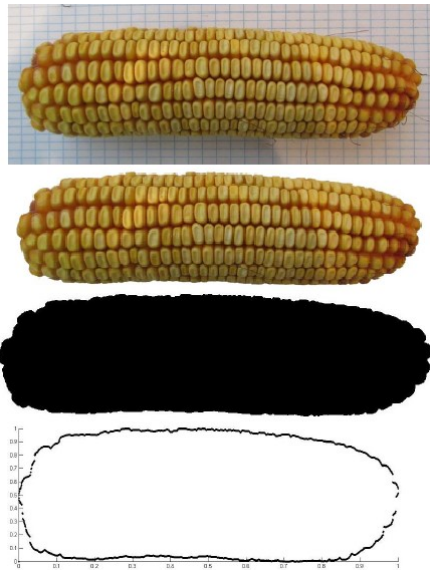
Figure 2: Image processing steps of corn ears shape
