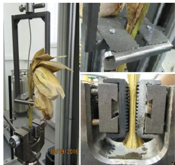
Figure 5: Apparatus for measurement of ear picking force
