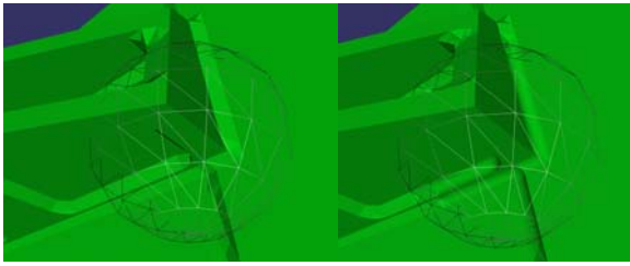
Figure 1 Adaptive meshing and local mesh refinements
