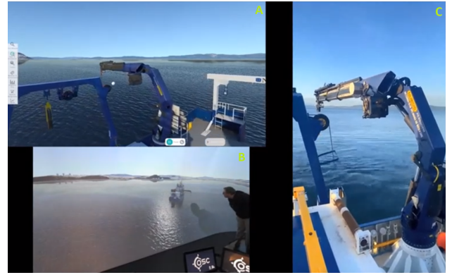
Fig. 7: A) Digital twin viewed from instructor panel, B) Visualisation the a stretched dome of the NTNU Ocean Space Lab, C) Live-feed from the ship during operation
