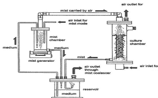
Figure 1: Flow Diagram Of Mist Reactor [11]
