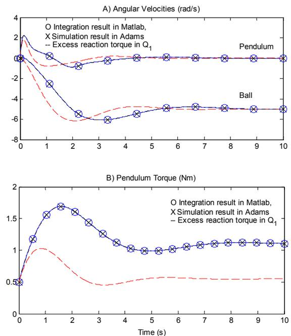
Figure 3: A) In a closed-loop, a PI-controller stabilizes the ball velocity. Excess reaction torque in  $Q_1$  causes a different system response. B) Excess reaction torque causes error in the simulated pendulum driving torque
