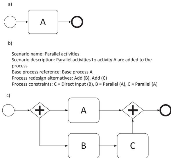
Figure 2: The base process modification example: a) base process; b) specification of the scenario; and c) a base process variant after applying the scenario specification rules
