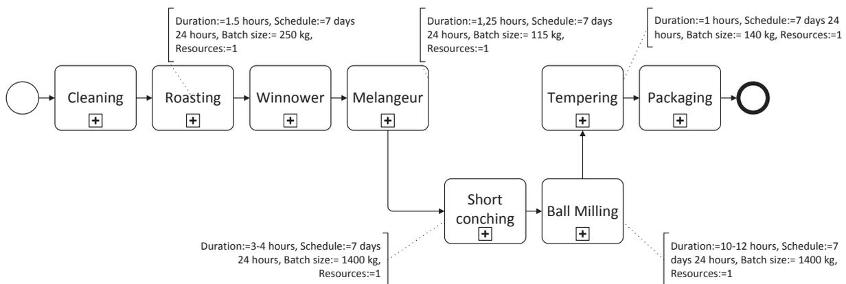
Figure 4: The process variant developed for scenario S4 with activity execution attributes
