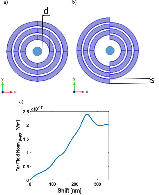
Figure 5: (a) Schematic illustration of a concentric grating structure with radial distance  $d = 500$  nm; top view. (b) Concentric grating with phase-shift  $s = 250$  nm. (c) Magnitude of the far-field in the forward direction ( $\theta = 90^\circ$ ) as a function of the phase shift  $s$ .
