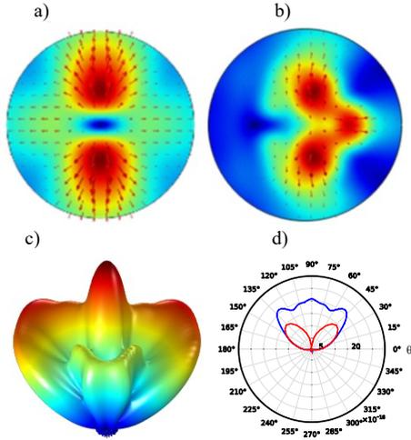
Figure 6: Magnitude of the SH electric field in the  $x$ - $y$  plane (top view) in the case of, (a), single cylinder, and, (b),  $N = 3$  grating. (c) SH far field in the  $y$ - $z$  plane in the case of  $N = 3$  grating. (d) Comparison of SH radiation pattern in the air region for pumping wavelength  $\lambda = 1710$  nm in the case of single cylinder (red line) and  $N = 3$  grating (blue line),  $y$ - $z$  plane.
