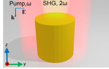
Figure 1: Schematic representation of SHG from a cylinder. The pump beam at  $\omega$  is a plane wave with wave vector,  $k$ , parallel to the cylinder axis.
