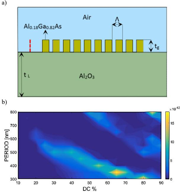
Figure 4: (a) Schematic picture of the system under study: one-dimensional high contrast grating realized in AlGaAs over an  $\text{Al}_2\text{O}_3$  low-index layer. (b) Scattered power as a function of grating period  $\Lambda$  and duty-cycle for a probe placed 1200 nm far away from the grating.
