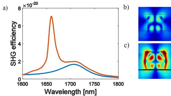
Figure 7: (a) Comparison of SHG efficiency in the case of single cylinder (blue line) and  $N = 3$  grating (orange line). (b) Normalized  $|E^{SH}|$  on a cross section in the  $y$ - $z$  plane at the centre of the cylinder without grating at pumping wavelength  $\lambda = 1710$  nm. (c) Normalized  $|E^{SH}|$  on a cross section in the  $y$ - $z$  plane at the centre of the cylinder with  $N = 3$  grating at pumping wavelength  $\lambda = 1710$  nm.
