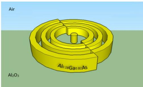
Figure 3: Schematic representation of the AlGaAs concentric grating over the  $\text{Al}_2\text{O}_3$  substrate.
