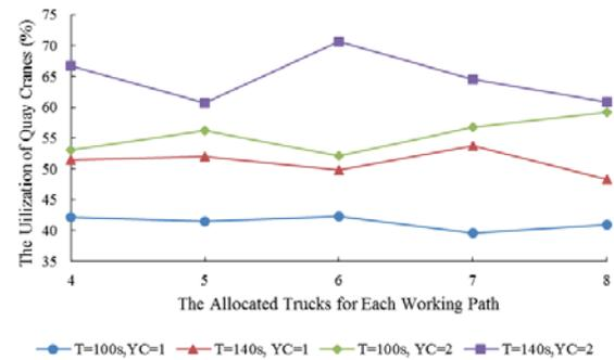
Figure 7: The Simulation Results of the Utilization of Quay Cranes
