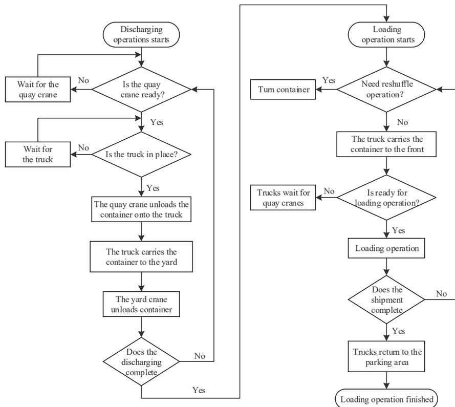
Figure 2: Flow Chart of Loading and Unloading Ship
