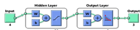
Fig. 2: Sorter ANN, a two-layer network with 20 sigmoid hidden neurons and 3 softmax output neurons.
