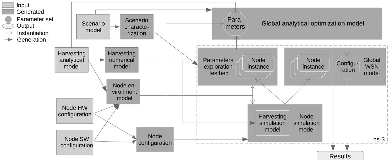
Fig. 2. The modeling and evaluation process
