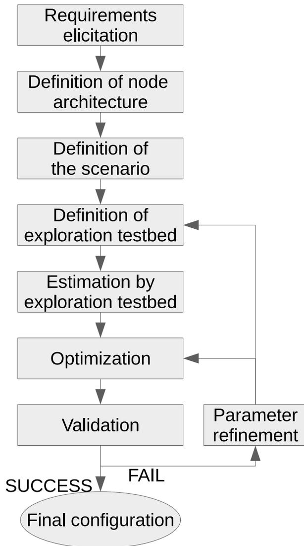
Fig. 1. The simulation methodology
