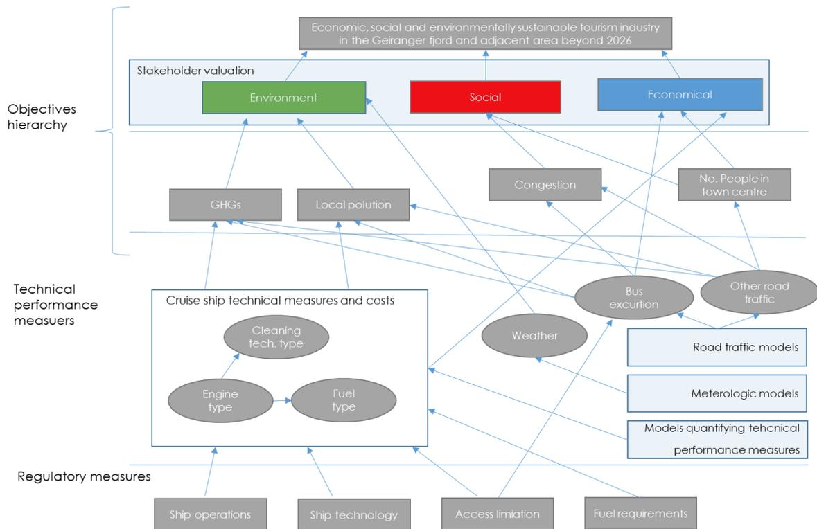
Figure 4: Example of Objectives Hierarchy, Technical Performance Measures and Regulatory Measures for Future Zero Emissions Sea Based Tourism Mobility in the Geiranger Fjord Area
