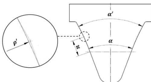
Figure 4. Modified rack-cutter tool profile
