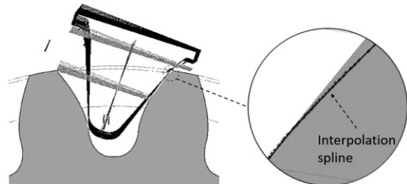
Figure 6. Interpolation splines of the modified profile
