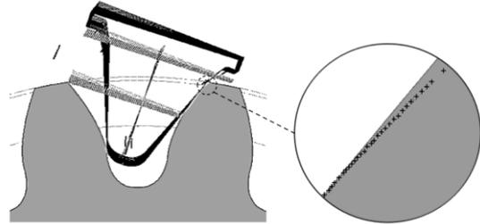
Figure 5. Intersection points of the tool edges
