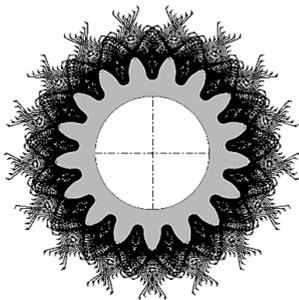
Figure 3. Tool paths of the original gear-cutter tool
