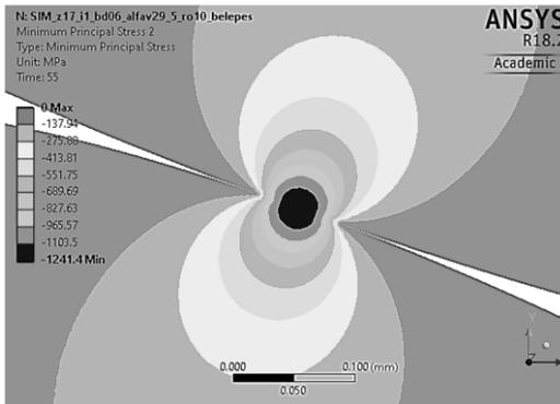
Figure 11. Minimum principal stress field of the gears
