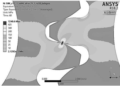
Figure 10. Equivalent stress field of the gear pair
