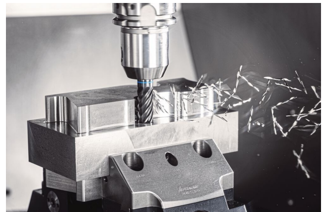
Fig. 1. In milling a moving and rotating tool with cutting edges removes chips from the stock and therefore forms the final shape of a work piece. [Image: Hoffmann GmbH Qualitätswerkzeuge]
