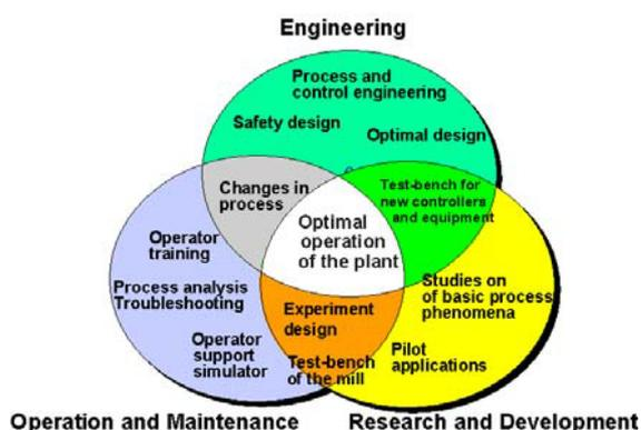
Figure 1: Role of a simulator in process industry
