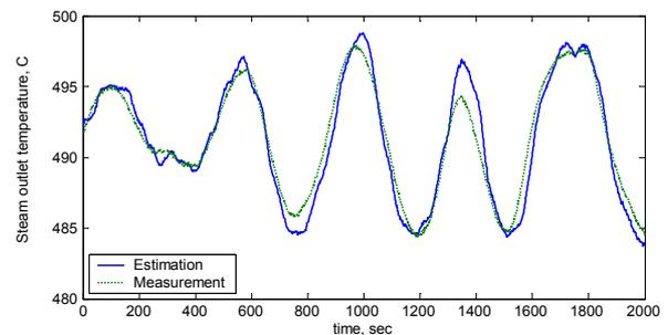
Figure 3. The measured and estimated outlet steam temperature in the identification
