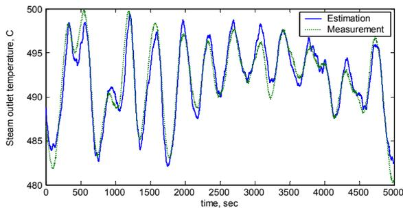
Figure 5. The measured and estimated outlet steam temperature in the validation
