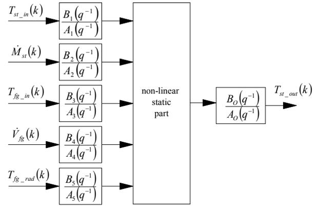
Figure 2. The Wiener-Hammerstein cascade model for the superheater
