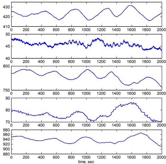
Figure 4. The model input variables (steam inlet temperature, steam mass flow, flue gas inlet temperature, flue gas volume flow, flue-gas representative temperature in the combustion chamber respectively) on the time range applied in the identification
