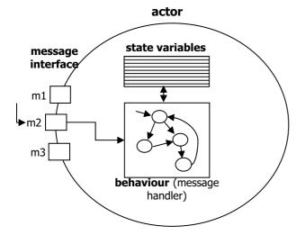
Fig. 1. Structure of an actor
