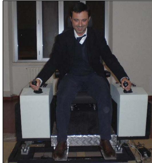
Figure 1: Mock-up motion platform
