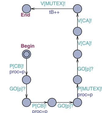
Figure 15. Automaton of B process
