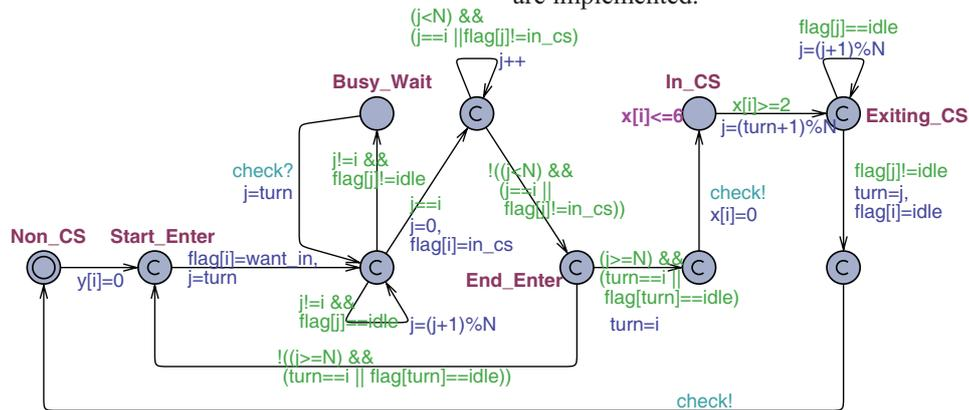
Figure 2. An UPPAAL Process template for Eisenberg and McGuire mutual exclusion algorithm
