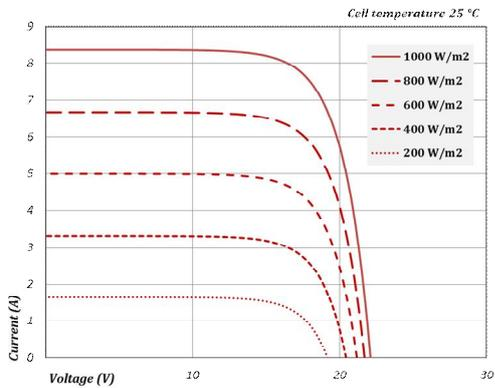
Figure 4: Calculated V-I Characteristics at Different Irradiancies with “Model 1”
