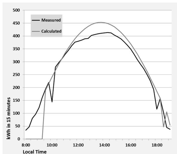
Figure 6: Comparison of the Measured and the Simulated Energy Produced on 10<sup>th</sup> July, 2013
