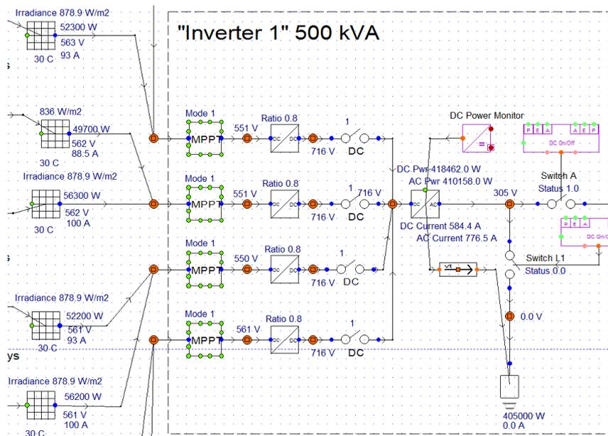
Figure 5: Part of a Model that Simulates a PV Production System Capable to 500 kW of AC Power.
