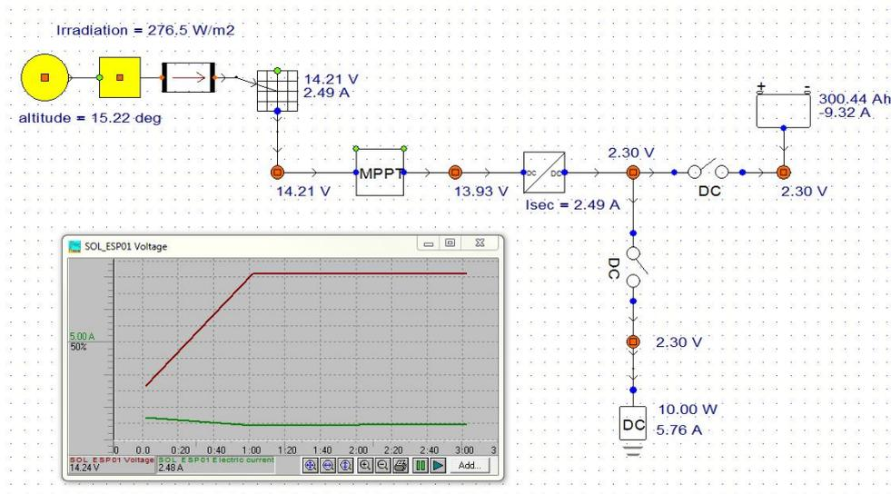
Figure 3: APROS Simulation of a Small-scale PV Energy Generation System
