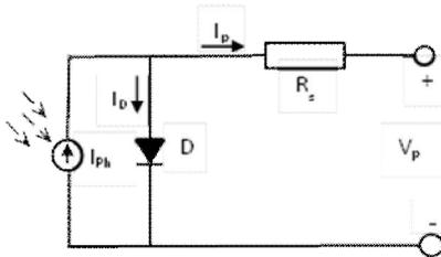
Figures 2: A Simplified Single-Diode Equivalent Circuit of a PV Module (Xiao et al. 2004; Bellini et al. 2009)
