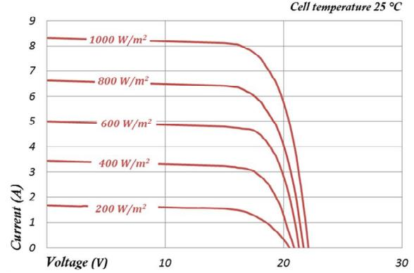
Figure 1: V-I Curve for A Typical Multicrystal Photovoltaic Module under 1,0 kW/m<sup>2</sup> Irradiation in Various Temperatures (on the left) and The Same Cell at T = 25° C under Different Radiation Intensities (Kyocera 2013)
