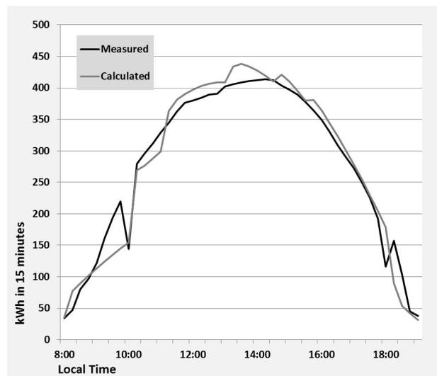
Figure 7: The Same Comparison as in Figure 6 when also the Changes in Cloudiness are simulated
