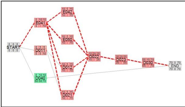
Figure 5: The PERT Network Diagram with the CP
