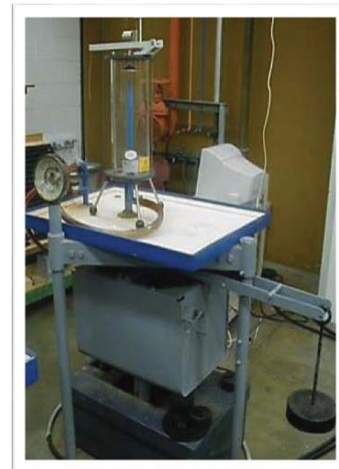
Figure 1. Physical Set-up of the Jet Force on Vanes Experiment
