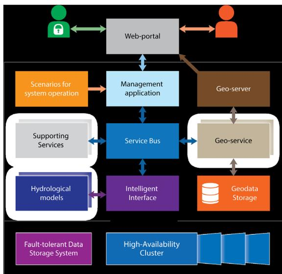
Figures 4. Structure of the system access to the results of flood monitoring and proactive modeling through Geo-portal.
