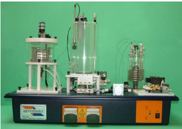
Figure 1: Basic Process Control Unit PCT40 with Process Vessel Accessory
