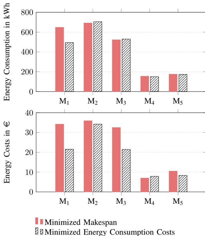
Fig. 2. Comparison of Schedule Plans in Terms of Energy Consumption and Costs
