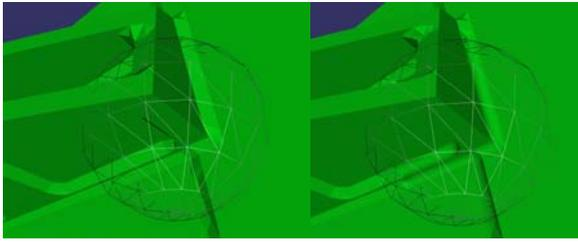
Figure 1 Adaptive meshing and local mesh refinements
