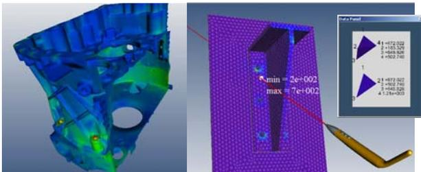
Figure 3 Interactive postprocessing of CAE data (left, mid: cross sectioning with clipping, right: element probing using laser beam metaphor)
