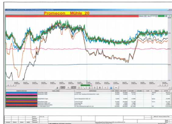
Figure 5: Implementation of the Kalman filter in Wilhelmshaven plant control system
