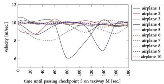
Figure 3: Speed-time plot of 10 airplanes taxiing on taxiway (Mazur and Schreckenberg 2018)
