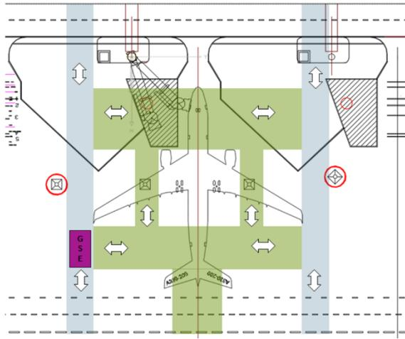
Figure 1: Proposed zoning and directions for GSE automated solution (Tabares and Mora-Camino 2017)
