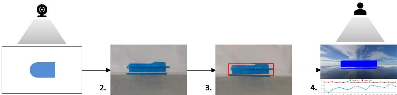
Figure 2: Data Gathering, Transmission, Processing and Usage for the Digital Twin of the Toy Boat
