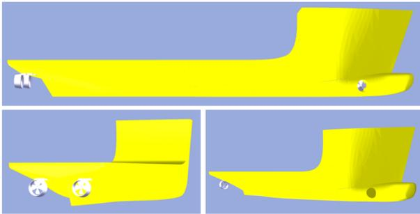
Figure 8: Visualization of the Ship Scale Model with DP System
