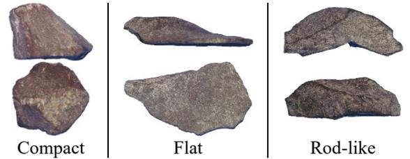
Figure 3: The Three Analysed Stones (Upper Images: Front View, Lower Images: Top View)
