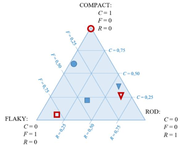
Figure 4: Shape Parameters of the Three Analysed Stones: Characterisation Based on the Surface Orientation Tensor: Hollow Circle  $\circ$ , Square  $\square$  and Triangle  $\nabla$  for the Compact, Flat and Rod Grains; Characterisation Based on the Overall Grain Shape according to Sneed and Folk (1958): Solid Circle  $\bullet$ , Square  $\blacksquare$  and Triangle  $\blacktriangledown$  for the Compact, Flat and Rod Grains Respectively
