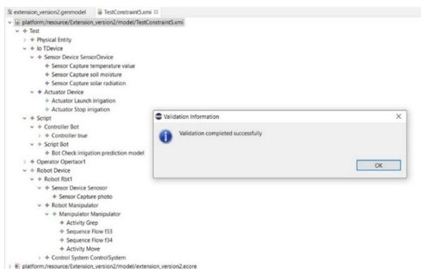
Figure 4: Validation of an agriculture IoRT-aware BP model using the *Selection Executor Constraints*
