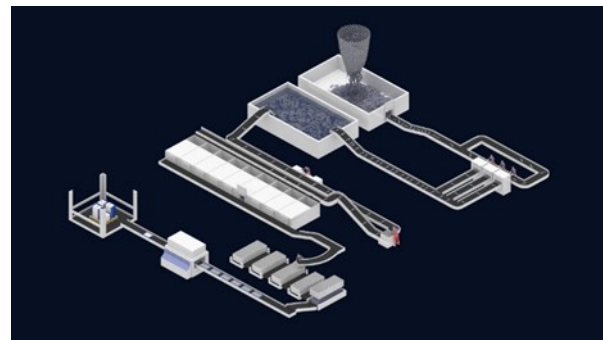
Figure 3: 3D Drawing of Processing Line for Headed and Gutted Fish on a Trawler
