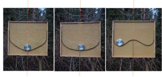
Figure 2. Model (made by Erazm M. Dutkiewicz) illustrating spontaneous symmetry breaking. Here the lost symmetry element is the mirror plane represented by the yellow trace.
