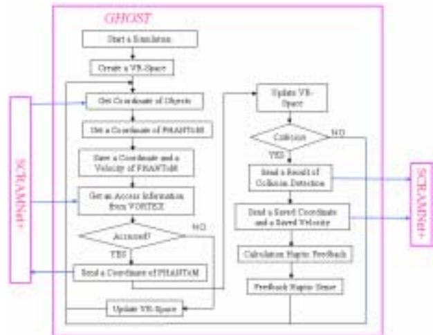
Figure 8: A flow of haptic system
