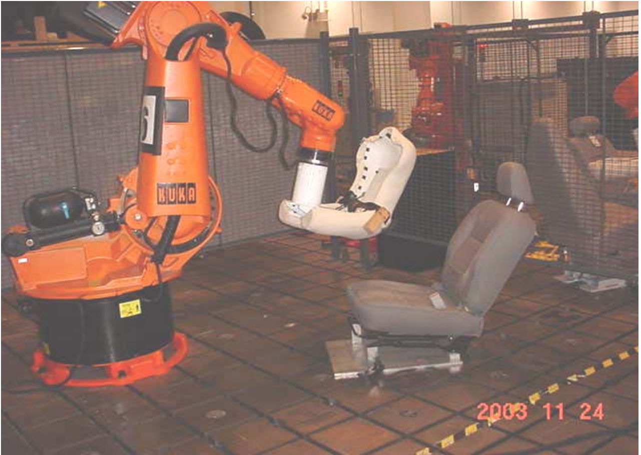
Figure 1. Robot, “Butt and Back Ford,” and Seat Under Test
