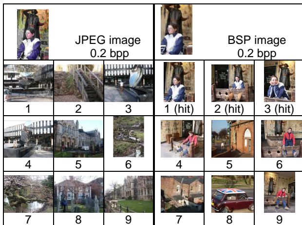
Figure 1: Example UCID query together with top 9 retrieved (using spatial-chromatic histograms) images both based on JPEG (left) and BSP (right) encoded images.
